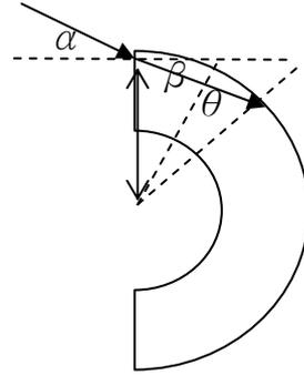
The bottom ray limits the maximum incident angle
